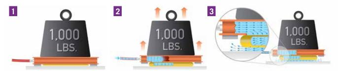
1. The red air hose feeds into a base module (orange) with an air caster (yellow) underneath. 2. Compressed air inflates the air caster and creates lift. 3. Excess air escapes the air caster, creating a film of air that floats the load like an air hockey puck.
