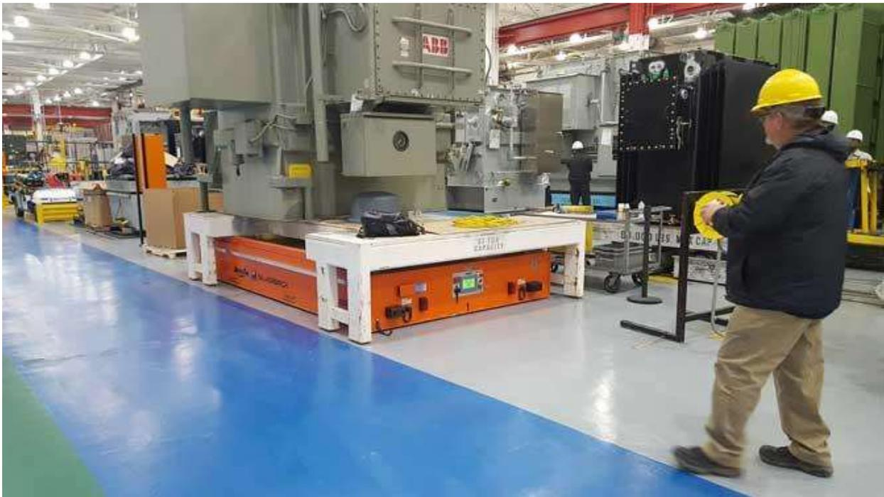
Manufacturers can safely transport loads up to 100 tons without damage to floors and with minimal manpower.
