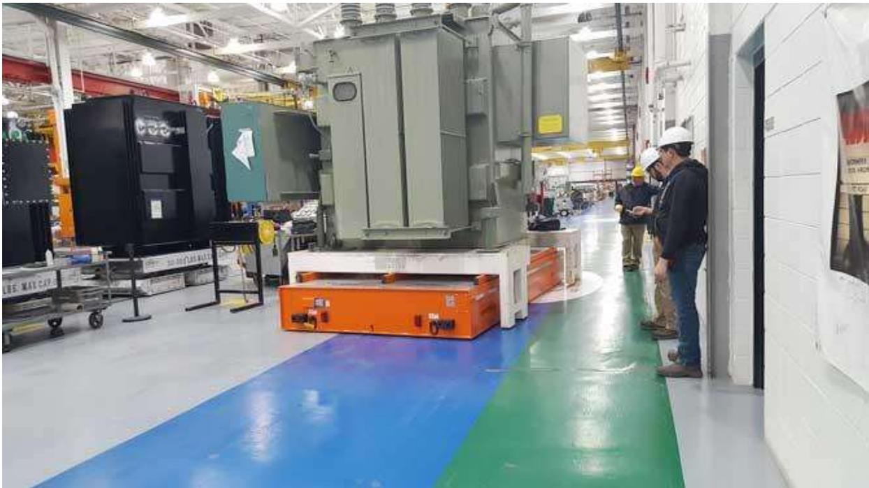
Self-Propelled Modular Transporters optimize factory floor space and production throughput.
