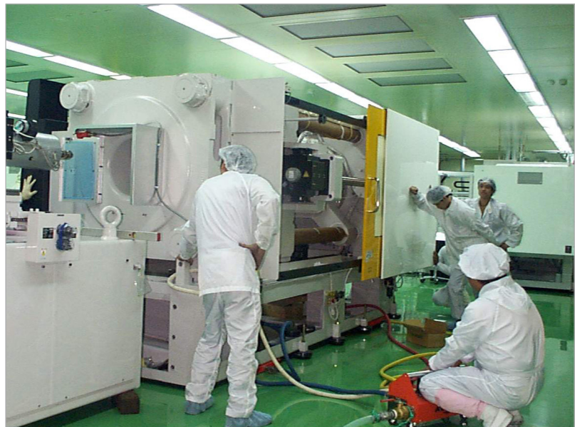
Manufacturers utilize all available floor space using air caster technology.
