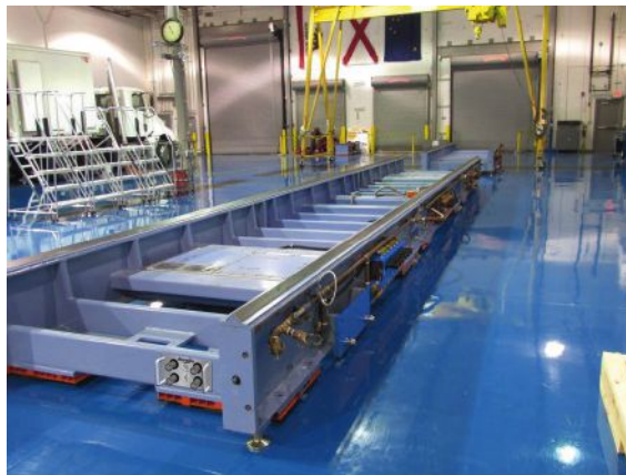
Figure 2: An embedded air bearing system permanently mounted into the tool, machine or structure serves as its own permanent rigging gear.
