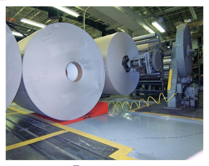
typically apply a protective layer, e.g. ultra-high molecular weight polyethylene, to act as a buffer between the loadmoving equipment and the paper roll.
